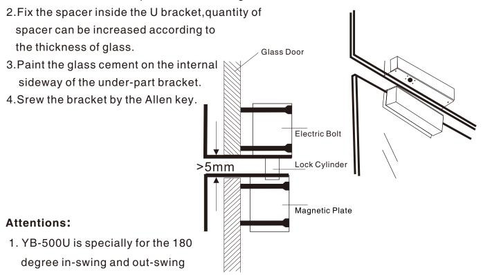
2. The thickness of glass door is 10-14mm
