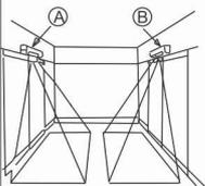
5.Please don't put it in place where the reflecting light such as sun light could reach the detecting lens, other wise it may cause error action.The back ground materials are marble and aluminum etc.
