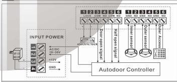
Note: When input voltage is DC12V, Please connect into POWER terminal 3 and 4. (as picture shown)
