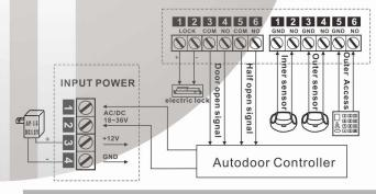
Note: When input voltage is DC12V, Please connect into POWER terminal 3 and 4.(as picture shown)
