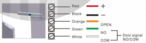
Under circumstance that two door are closed correctly by detection, lock will release signal
