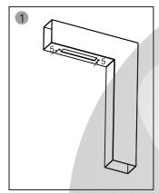
Incise the location of face plate and magnetic plate in the door leaf and door farme according to the mark of lore size
