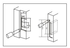
2. Accrding to the painting, use the propertools to drawthe relative hole and mortise groove on the door and door frame.
