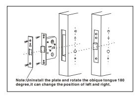
5.Install the knob of decorative panel with button, and check whether it is saftly or not, and the handle should be make the oblique tongue flexible, and fasten two screws of decorative panel, then fasten the handle with fixing-screws.
