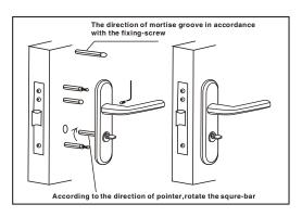
Warning: A. The direction of mortise groove in accordance with the fixing-screw when install the squar-bar. B.Lock body should be in a insafety condition, then the oblique tongue can flex freely. C. Draw the key when install the decorative panel, according to the direction of lock tongue, rotate the small squre-baroppositely direction of to the end. Then you can put the small squre-bar into the small squre-hole of lock body. Or you can not draw the key and close the door.
