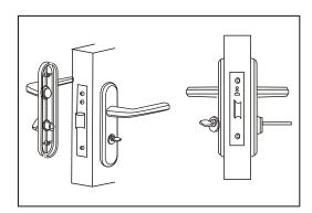
7. After all ofthose, check the doorlock, it must be flexible; handle need runningsmoothly when we rotate; it's useful with key whenopen; rotate-button is flexible, if everything is ok, please fix all of the screws tightly.
