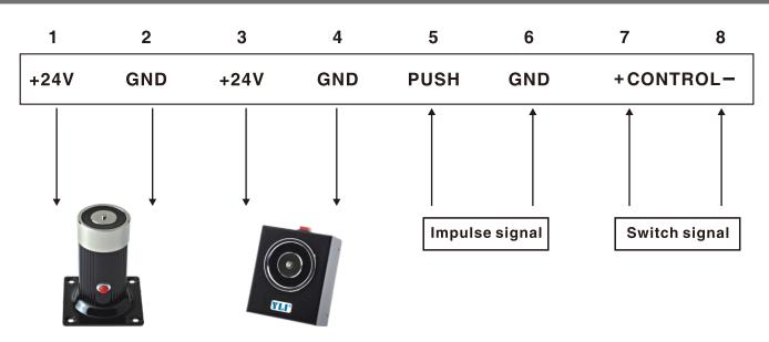
1-2 and 3-4: 1-2: DC24V output, 1&3 are positive electrode and 2&4 negative.
